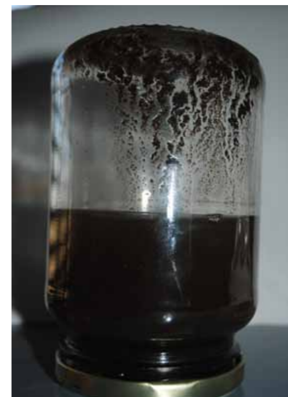
Coal particles from a patch of roof washed approx half a kilometre from coal train line. Queensland
